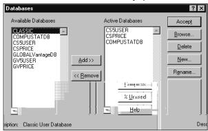
This is the primary dialog box used for database management within the Research Insight application; it includes a listing of all Available Databases, a listing of all Active Databases in the group and buttons enabling you to add, delete, rename and compress databases. Each option is covered in detail in a later section of this chapter titled, *Moving atabases from One Group to Another*. For now, we'll use it to create a new database.
